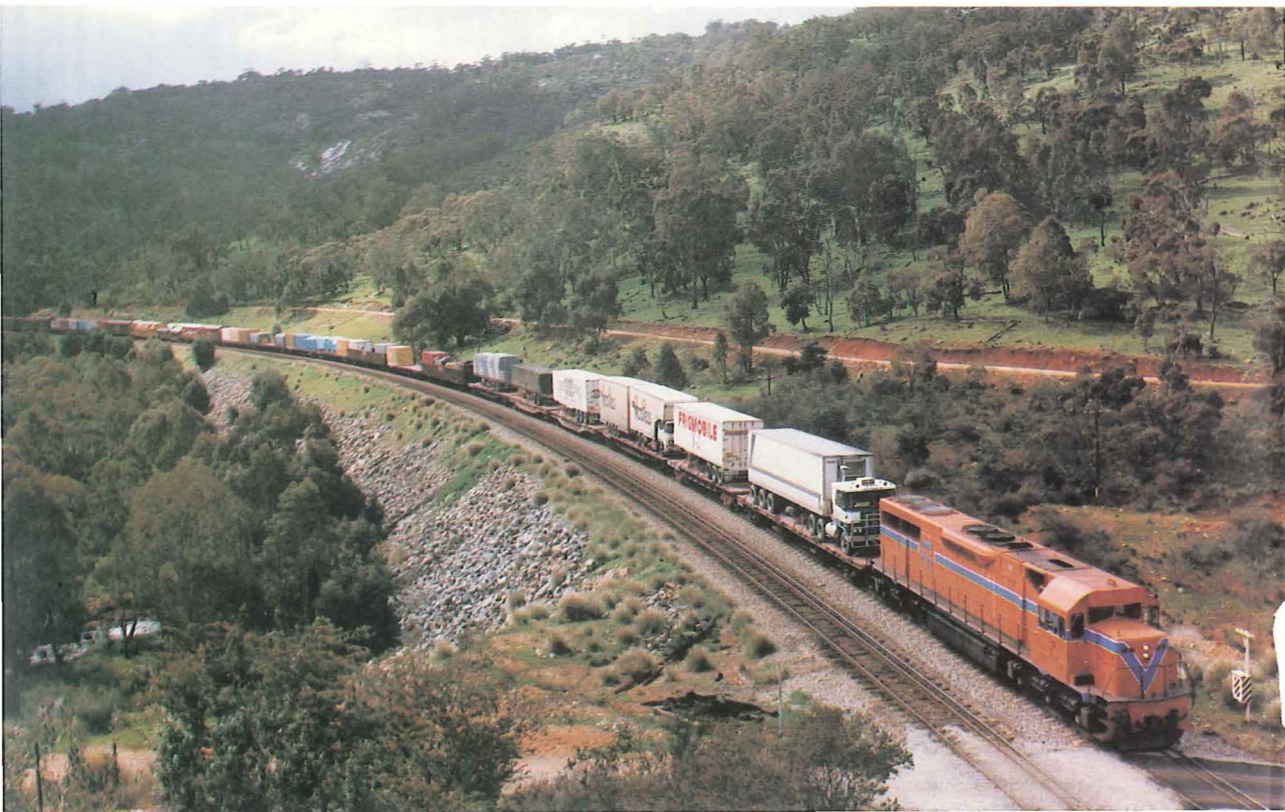
PLATE 14 — A 3,300 HP 'L' Class Westrail locomotive pulling a load of westbound piggyback, container and general freight, through the Avon Valley.
